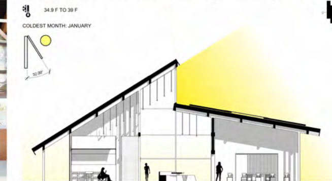
HEATING IN WINTER- TRANSVERSE SECTION
