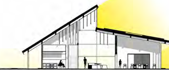
HEATING IN WINTER- TRANSVERSE SECTION
